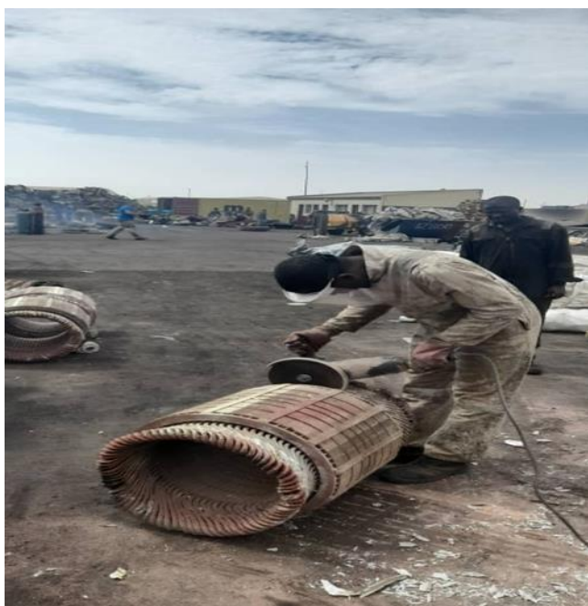
Photo 5. Workers cutting scrap metal using grinder. Photo 6. Gas bottles in use
